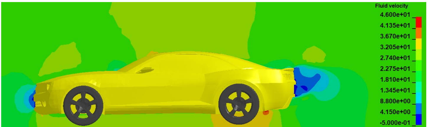
Figure 14 : Fluid velocity for the initial design
