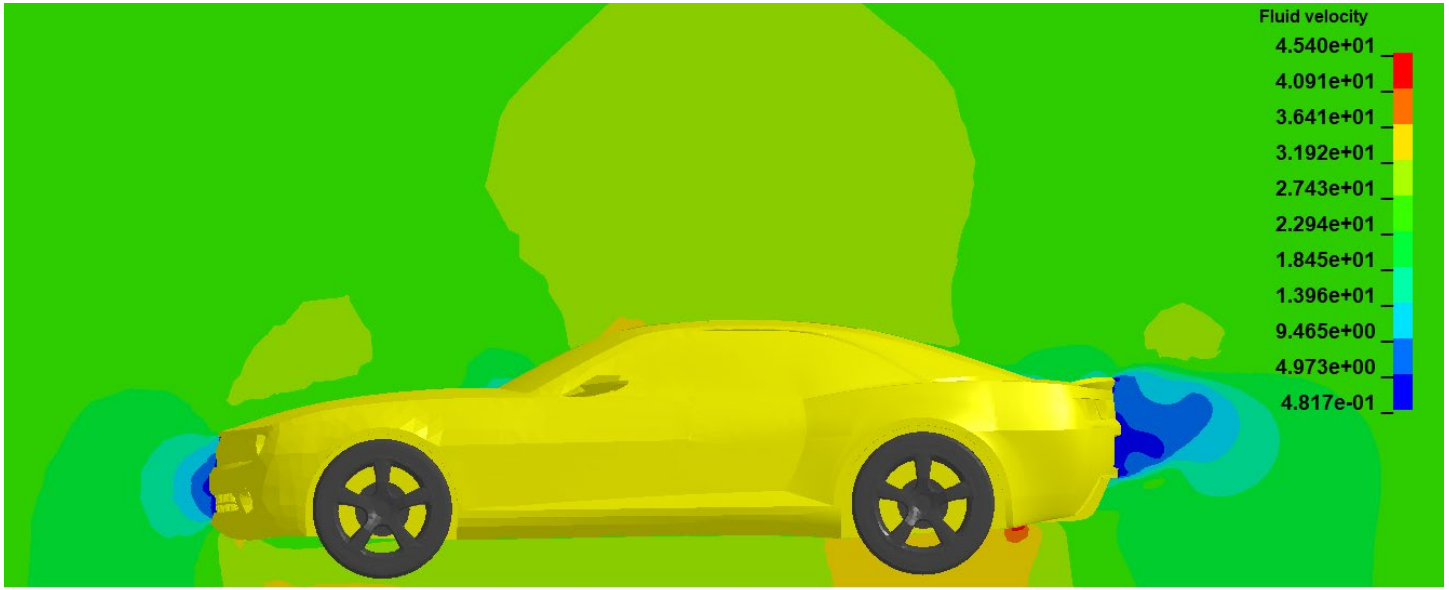
Figure 9 : Fluid velocity on the initial design
